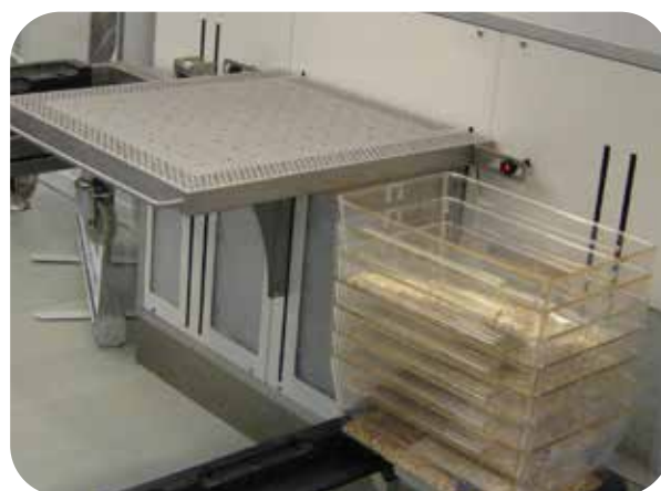
Optional: Automatic dispensers on each side of the height adjustable, perforated table.
